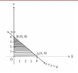
The shaded region (OAB) in the above figure is the feasible region determined by the system of constraints  $x \ge 0$ ,  $y \ge 0$  and  $x + y \le 4$ .
